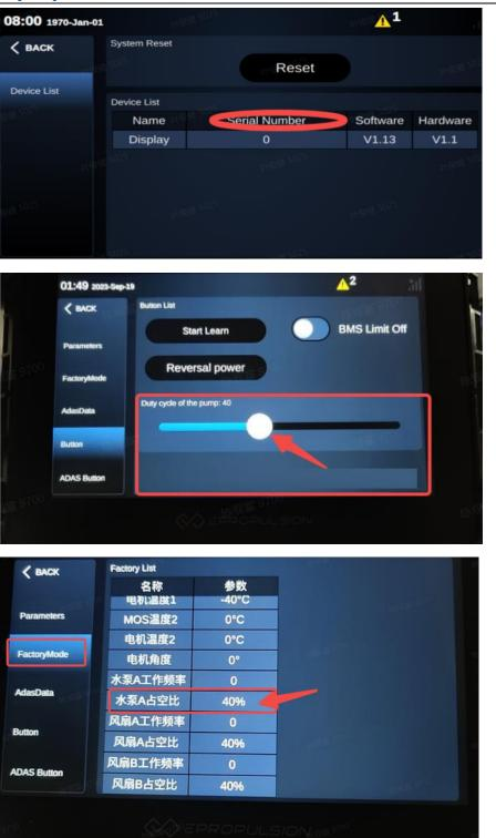
During the operation of the water pump, continue to add coolant and inject a total of 1550mL, as there may be deviations in the length of the pipeline cutting. The entire process may take up to 5 minutes. Due to the previous injection of coolant into this machine, it may not be able to drain completely. If 1550mL cannot be fully injected, continue to add coolant to maintain the liquid level on the upper edge of the filter screen.
