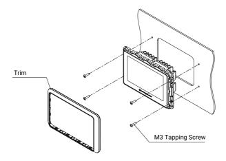
4 Put the display trim back on the display and press it in place of the four corners so that the trim is flush with the display.
