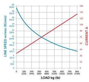
The motor will cut-out at pre-determined current and temperature limits.
