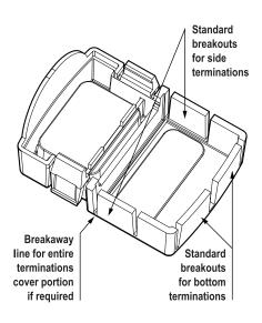
Standard breakouts allow wire access from sides and bottom directions.
