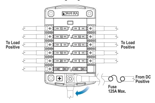
Application Note: This device is intended for branch circuit protection. Suitable main circuit protection of not more than 125A rating should be provided ahead of this device with an interrupt current rating consistent with the battery capacity. Consult ABYC E-11 Table V See "Circuit Protection" at www.bluesea.com.
