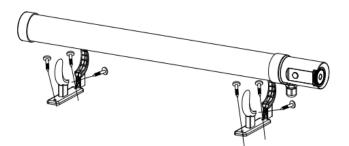
Step 2. Fix the tubular heater on the wall or on the floor like the following picture showed .
